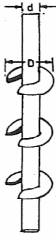
Figure 3 The schematic drawing of the screw pile with three helix plates. The helix plate diameter D ranges typically from 150 mm to 600 mm and the shaft diameter d ranges typically from 60 mm to 140 mm
